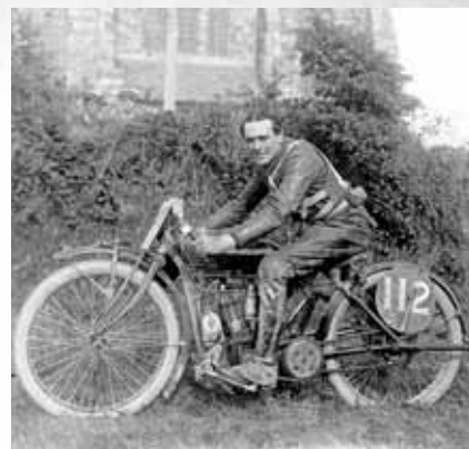
The displacement limit for twin-cylinder bikes competing in the 1911 Senior TT was 580cc. Indian had to sleeve down its 750cc "Little Twin" to qualify for the event.
