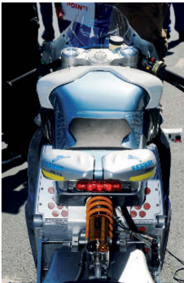
Left: Quick-change battery system on Miller's 2010 bike. Below: battery bulk – the big problem with electric bikes. A rumoured 285kg is five stone more than a ZZ-R1100
