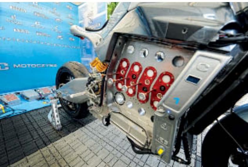
Left: Quick-change battery system on Miller's 2010 bike. Below: battery bulk – the big problem with electric bikes. A rumoured 285kg is five stone more than a ZZ-R1100
